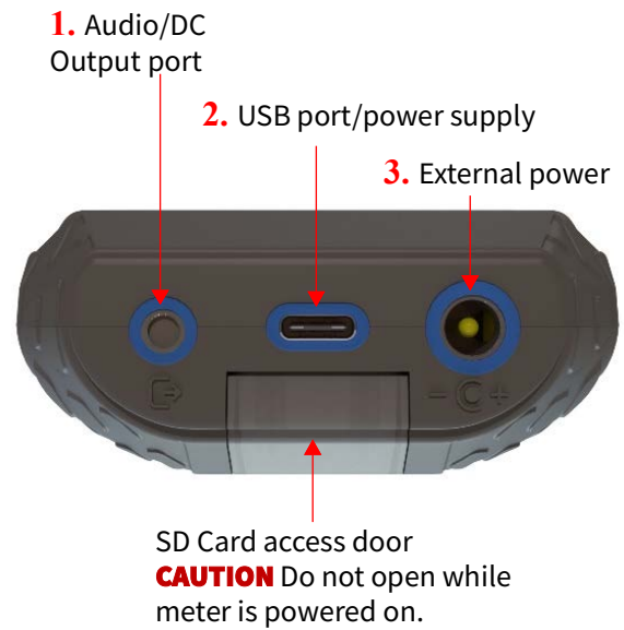
FIGURE 1-2 Main Body: Bottom Connectors
